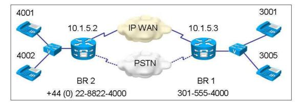
In this scenario, Branch 1 has moved. The area code is the same, but the main number for the office has changed, although the extension numbers remain the same. Calls from Branch 2 to Branch 1 can still use 4-digit dialing over the IP WAN, but calls that are placed over the PSTN now fail because the DID range is different from the extension numbers.
