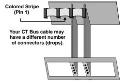
3. If the cable has extra connectors or is loose, tuck the cable down so that it does not snag when you replace the computer cover. See the **Caution** given earlier in this section.
