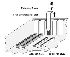
**Note:** If you are not installing your board in an ISA form-factor PCI slot, remove the slot retainer bracket from the end of the board before installation.
