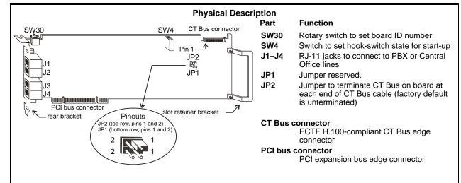
3. Insert the board's edge connector into the bus slot. Use the slot's board guides as you insert the board edge connector into the slot. Apply pressure only to the top edge of the board, and press firmly until the edge connector is securely seated in the slot.
