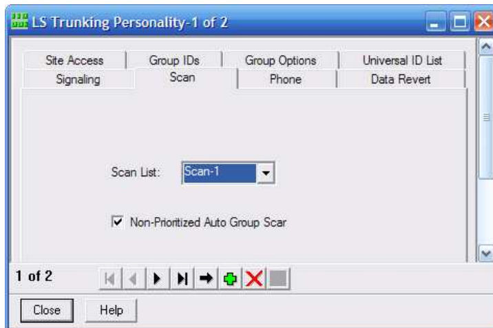
Figure 3-7 LS Trunking Personality/Scan – Scan List refers to a System Scan List that can be chosen for the each LS Trunking Personality. When the Non-Prioritized Auto Group Scan box is un-checked, the radio will perform Prioritized Auto Group Scan, when enabled, on the groups selected for Auto Group Scan in the Group Options window. Auto Group Scan and the Scan List are not related features.
