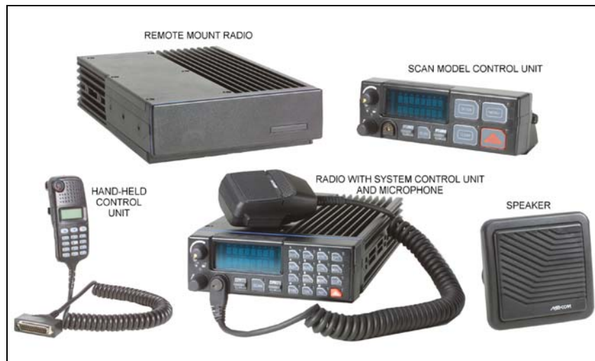
Figure 1 – M7100 IP Series Mobile Radio Components
