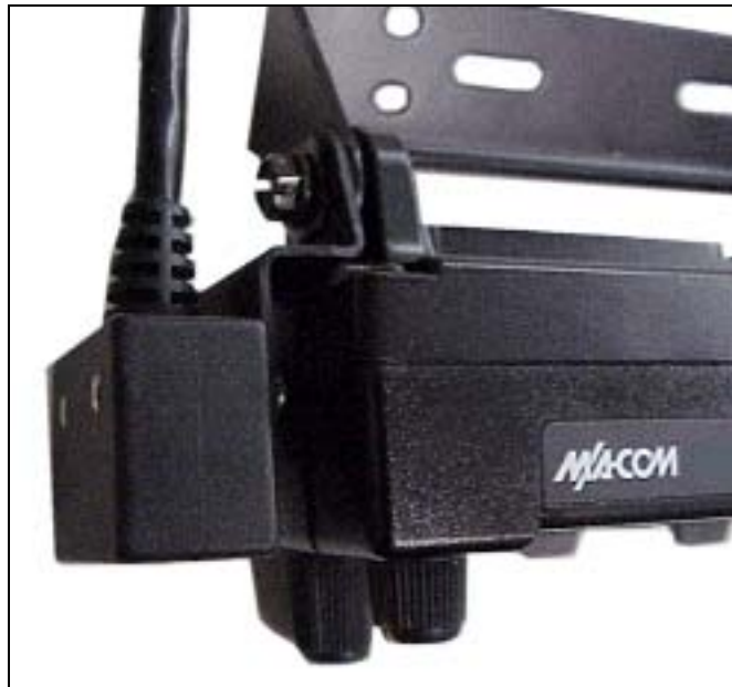
Figure 15 – Pigtail Bracket Installed on Control Unit
