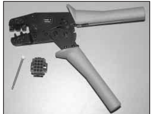
The supplied crimp tool (with extractor pin) is used to wire up all I/O connector plugs.
