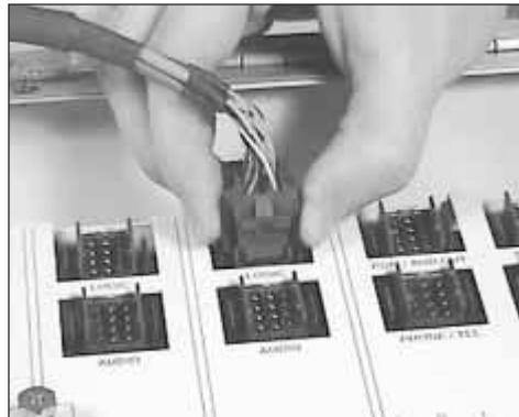
Close-up of a wired-up 12-pin I/O connector plug being inserted into its PCB-mounted socket.
