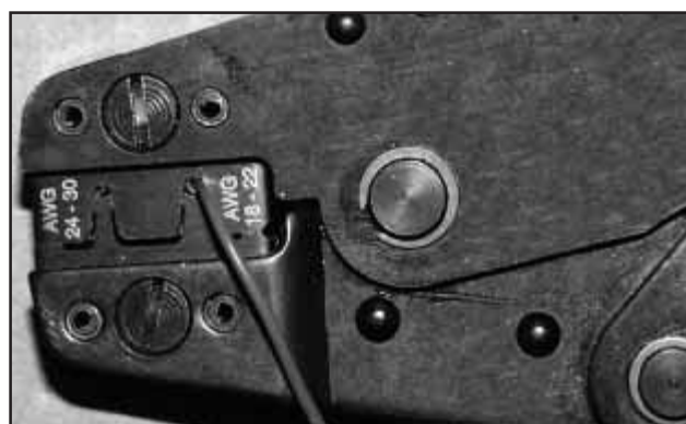
(4) Final step: jaws fully closed; the insulation tabs have been crimped.
