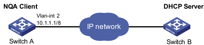
Figure 310 Network diagram for DHCP
