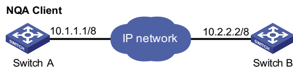
Figure 309 Network diagram for the ICMP-echo test
