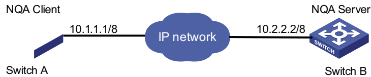
Figure 313 Network diagram for UDP-jitter test
