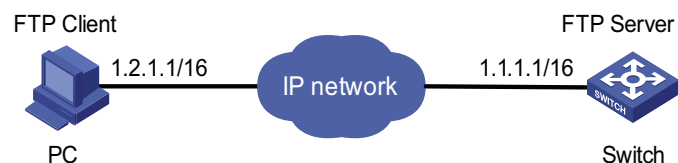
Figure 299 Smooth upgrading using the FTP server
