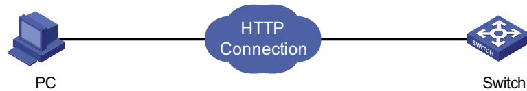
Figure 19 Establish an HTTP connection between your PC and the switch
