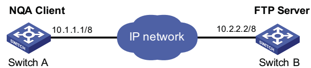
Figure 311 Network diagram for FTP
