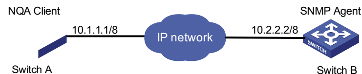
Figure 314 Network diagram for SNMP test
