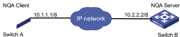
Figure 315 Network diagram for the TCP test
